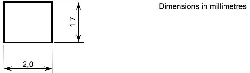
Figure 1 — Minimum dimensions of the contacts
