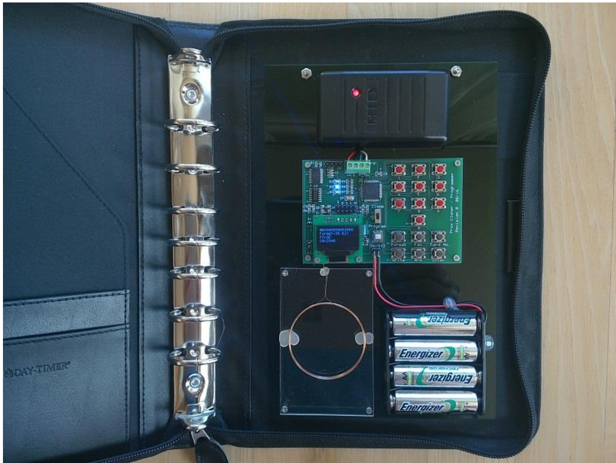
Cloner/Programmer Circuit installed into a “Covert” Day Planner Notebook
